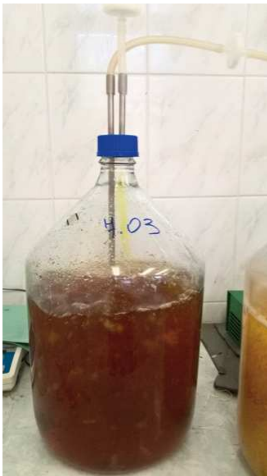
Fig.1. Air-lift system for mushroom biomass production
