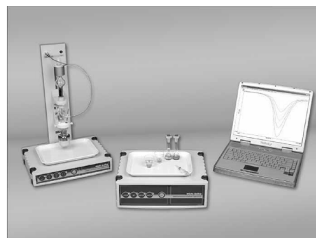
Fig. 1 Typical Polarographic/Voltammetric analyzer – MTM Anko; (M161 Analyser), (M164 CGMDE – Controlled Growth Mercury Electrode – Stand)
